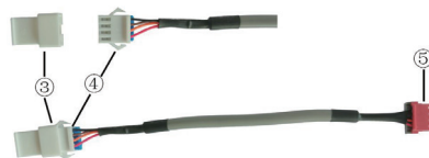
Fig. 4.6.5: Schematic diagram of patch cord: Terminal ③ is the protection terminal; connect terminal ④ to the terminal ② of connection wire; connect terminal ⑤ to the terminal of wired controller of air conditioner
