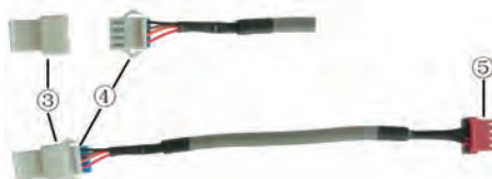
Fig 32: Schematic diagram of patch cord: Terminal ③ is the protection terminal; connect terminal ④ to the terminal ② of connection wire; connect terminal ⑤ to the terminal of wired controller of air conditioner
