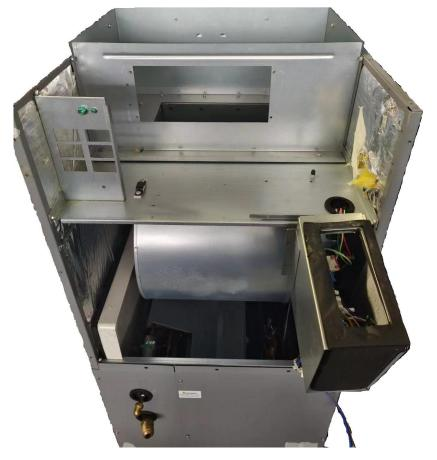
4. Install the electric heater in the position of the metal plate removed at Step 3. (Note: There are two holes underneath. They are used to fix the bracket of the electric heater.)
