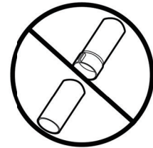
Do not crimp service valve connector when pipe is smaller than connector
