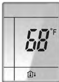
Room Temperature Display
