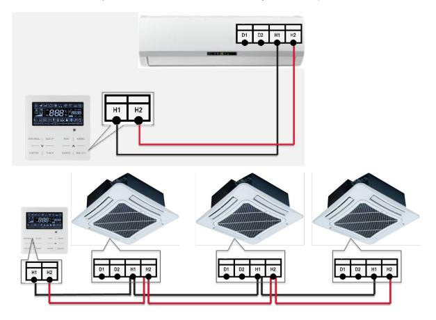
• Controller needs to be set to control multiple units. Refer to Controller Installation Instructions.
