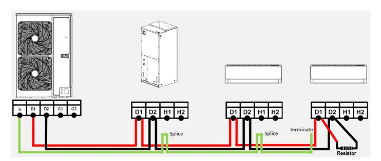
120 ohm 1/4 watt resistor is shipped with outdoor unit and is connected at the last indoor unit
