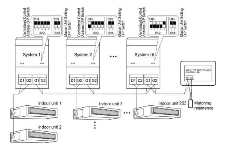
1 = OFF 0 = On Dip switches are located on the main board of the condenser Address one is default, all dip switches on.
